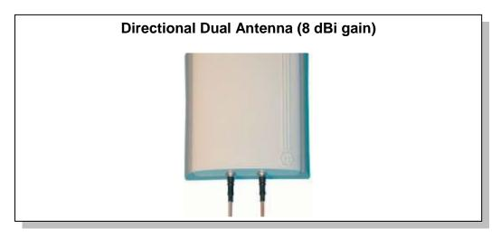
The 'directional dual antenna' consists of two flat directional antennas housed in a plastic shroud. It is fitted with 1 meter of coaxial cable and a MCX male connector. The antenna includes a side tilt and a wall bracket by which it can be adjusted in a horizontal plane. The antenna can be mounted to a pole of 40 to 90 mm in diameter by means of a steel strap (included).
