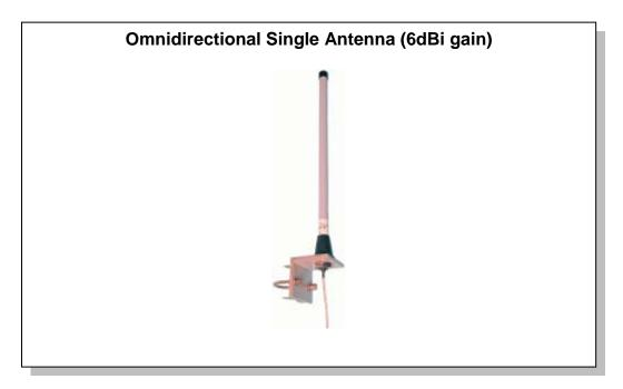
The 'omnidirectional single antenna' is an omnidirectional 6 dBi colinear antenna fitted with a 1 meter coaxial cable and a MCX male connector. It is supplied with a wall bracket and a pole mounting clamp. With this pole mounting clamp the antenna can be mounted to a pole with diameter of 25 to 37 mm.
