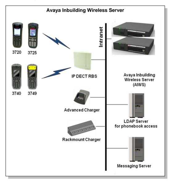
The Avaya Inbuilding Wireless Server (AIWS) is a Linux based appliance server that adds additional value to the DECT R4 solution. It is an optional component and neither mandatory for the installation nor for the operation of a DECT R4 system. The additional functions provided by the AIWS server are as follows:
