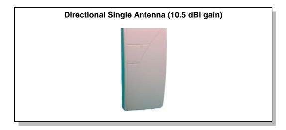
The 'directional single antenna' is a flat directional antenna housed in a plastic shroud and fitted with 1 meter of coaxial cable and a MCX male connector. The antenna includes a rotating bracket for wall installation. It can be adjusted in both a vertical and a horizontal plane. The mounting bracket allows installation by strapping
